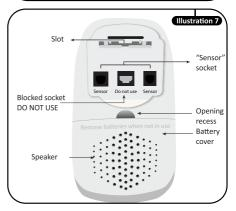
8. Press control unit holder or hanging hook firmly into slot in back of control unit (see illustration and 7).
