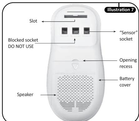
8. Press control unit holder or hanging hook firmly into slot in back of control unit (see illustration 6 and 7).
